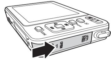
To remove the SD/MMC/SDHC card, gently push the card until it pops out. Pull out the card carefully.
